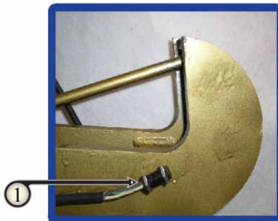
\*Note: Switch mounted internally under the hook
